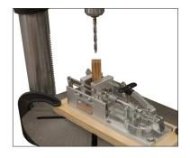
Drill the pen blank with a 27/64" drill bit.
