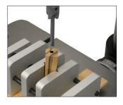
Using a sander or barrel trimmer, square the ends of your pen blank so that it is flush to the ends of the tube that is inserted into the pen blank. When squaring the ends of your blank, do not remove any of the brass. Removing any of the brass tube will change the overall length of the finished pen which will affect the overall operation of the pen.
